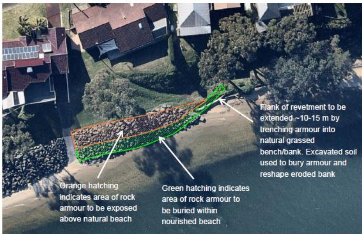
Figure 2. Proposed concept design solution to ameliorate the end effect erosion.
