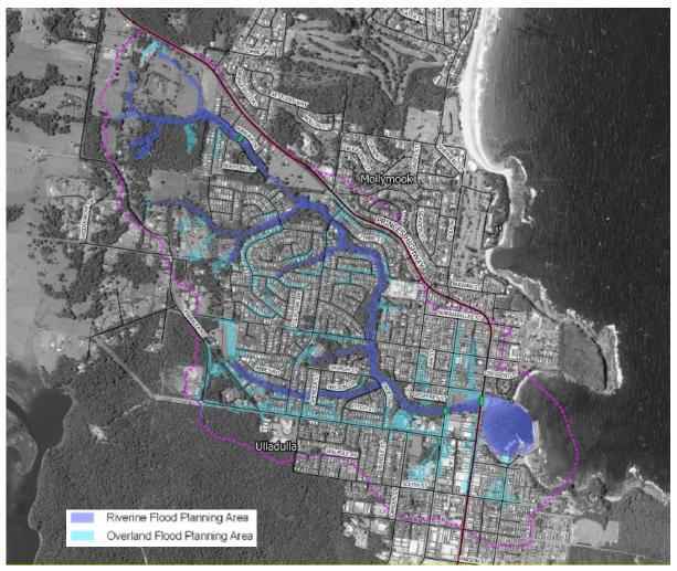
Figure 1 Millards Creek Catchment – Riverine and Overland Flood Planning Area (Source: Draft Millards Creek Flood Study).
