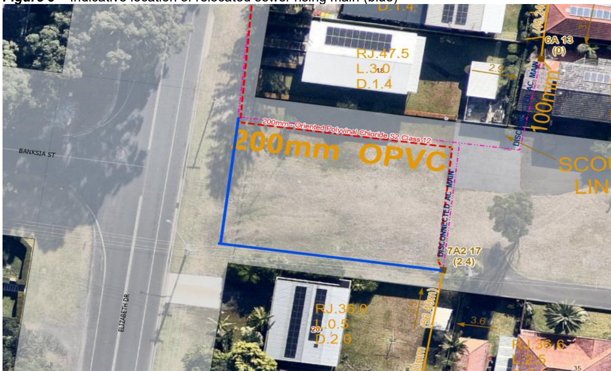
Figure 3 – Indicative location of relocated sewer rising main (blue)
