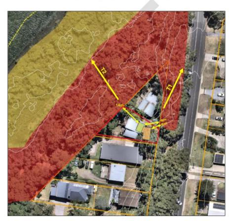
Figure 5: Effective slope analysis (Nearmap/LIDAR 1m Contours) showing setbacks from hazard.
