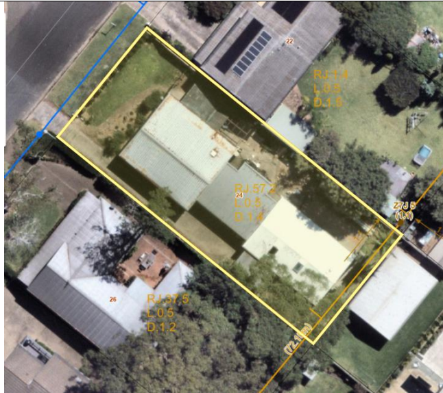
Figure 3 - Council reticulated Sewer and Water Services available to the subject site and both existing developments (blue representing water lines and yellow representing sewer lines)
