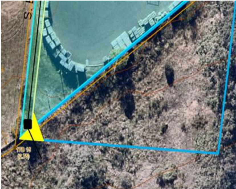
Figure 3: Indicative sketch showing approximate location of existing drainage infrastructure in black and approximate proposed drainage easement location highlighted in yellow.
