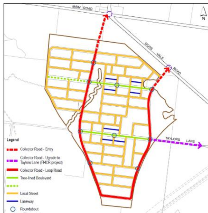
Figure 2: Street Hierarchy and Network Plan (DCP Chapter NB3)
