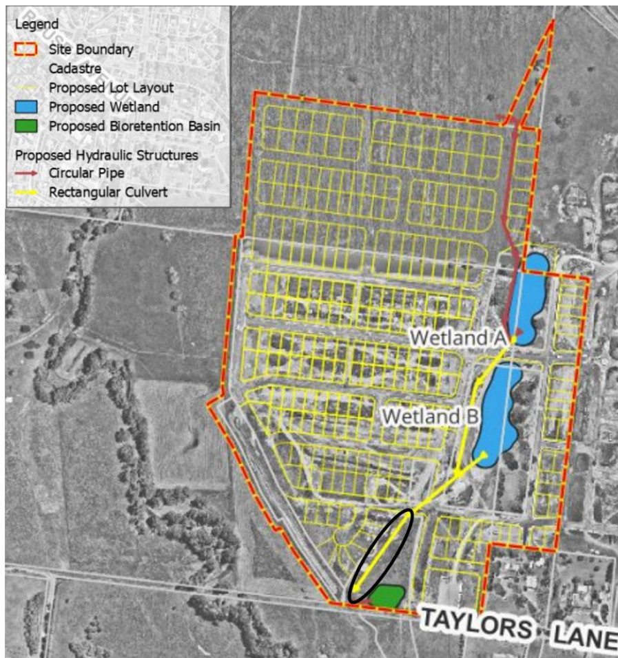
Figure 2: Location of drainage infrastructure Wetland A, Wetland B, Bioretention Basin and the portion of culvert circled black
