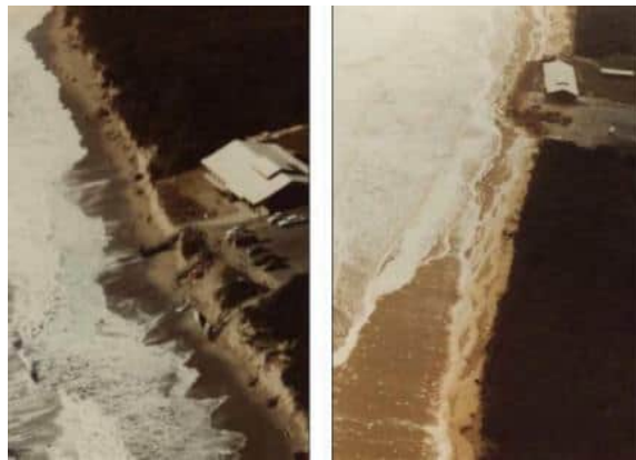
Figure 2-2 Shoalhaven Heads Beach showing Surf Club in 1977 (left) and following rock protection in 1978 (right). Image source: DCCEEW.
