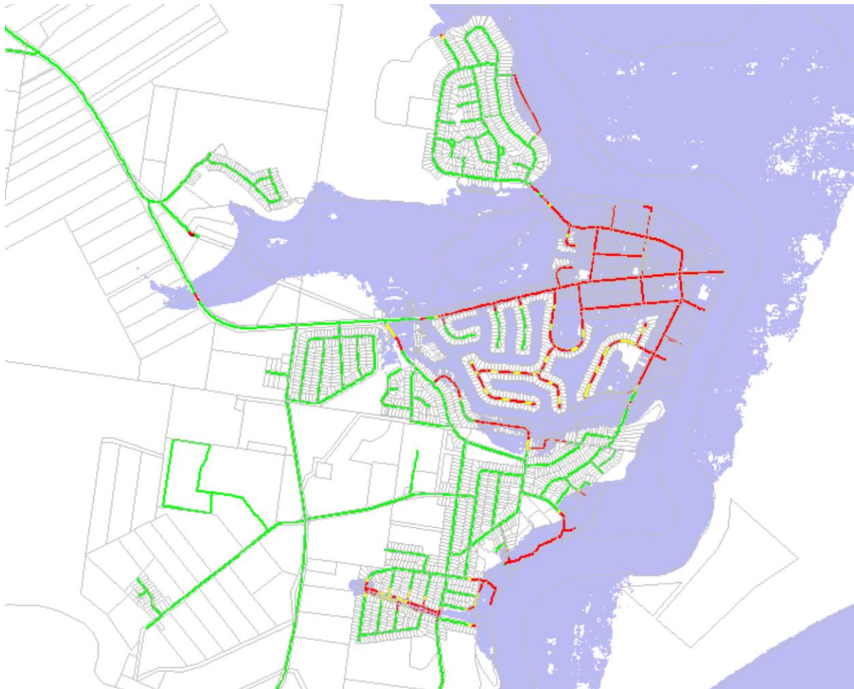
Figure 1 Road Inundation at Sussex Inlet in 1% AEP Event ('green' is flood free, 'yellow' is potentially inundated but to less than 0.3m deep and 'red' is inundated to a depth greater than 0.3m)
