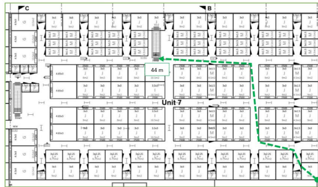
Figure 10: Diagram of the DtS deviation (Unit 7 First Floor)
