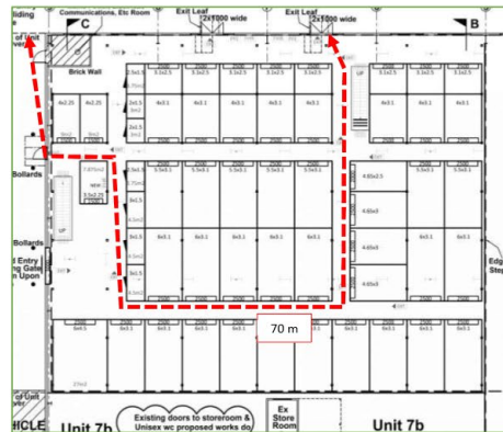
Figure 9: Diagram of the DtS deviation (Unit 7 Ground Floor)
