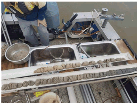
Figure 6-1: View of split sediment core on the sampling vessel, allowing visual examination of the material to be dredged, logging, photography and subsampling for laboratory testing
