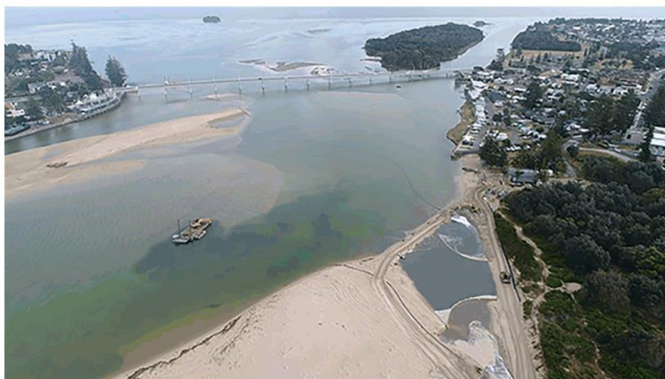
Figure 4-7: Aerial oblique view of The Entrance showing the dredger working in the channel and pumping to a settling pond (lower right)
