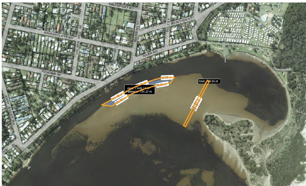
Figure 5: Map showing proposed dredged navigation channel and proposed dredged sand bar to provide wider bank buffer
