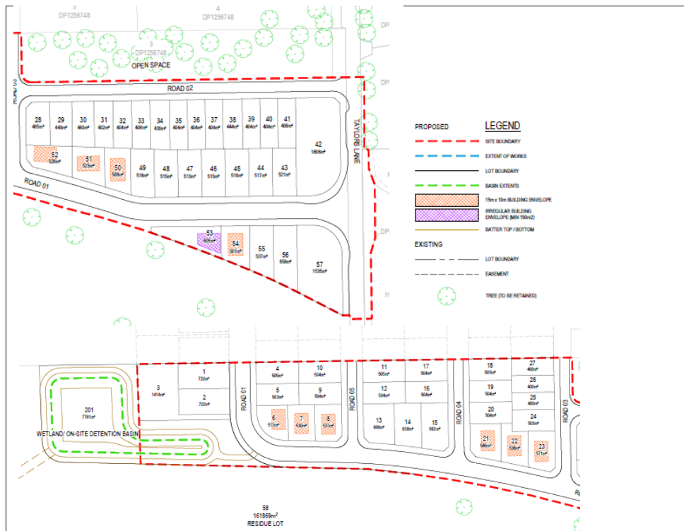
Figure 5 – Non-Compliant Lot Building Envelope Layout Plan by Maker ENG within Design Verification Statement (dated 19/07/2021)
