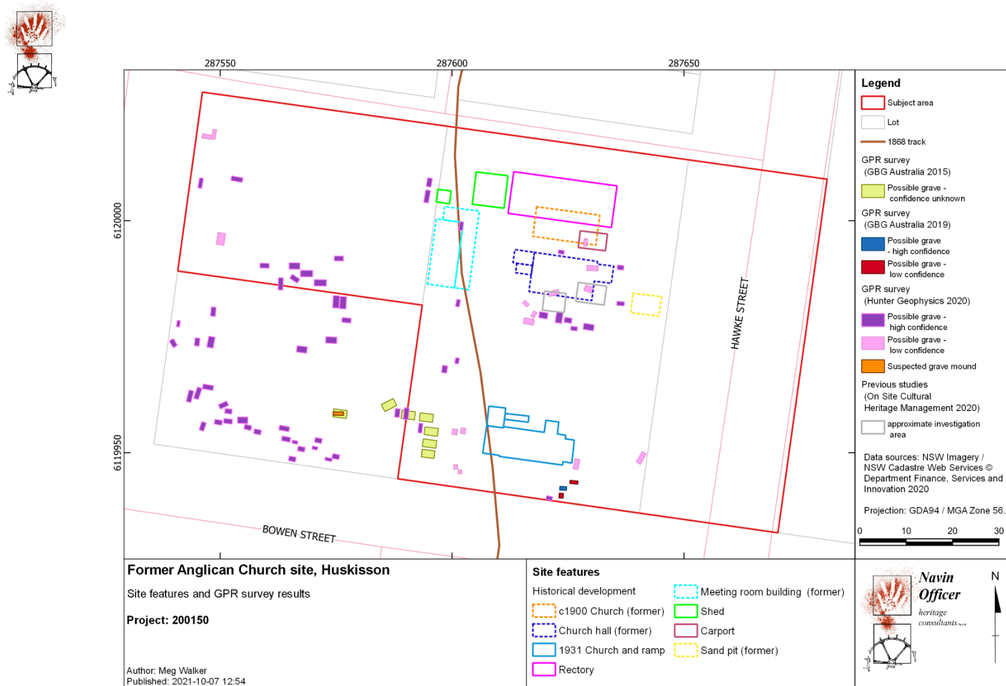
Figure 5-8 Results from the GPR survey conducted by Hunter Geophysics (2021:26) at the Former Anglican Church site in Huskisson. Purple units are anomalies that met the criteria selected to match possible graves and light pink units represent anomalies that met some but not all of the criteria selected.
