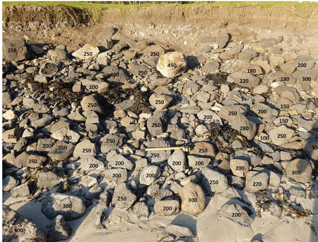
Figure 3 – Representative sample for estimated diameter of existing rock on site, annotated with estimated diameter
