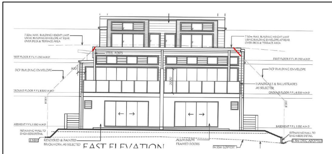
Figure 2 – Eastern elevation showing encroachment beyond Chapter G6 building envelope
