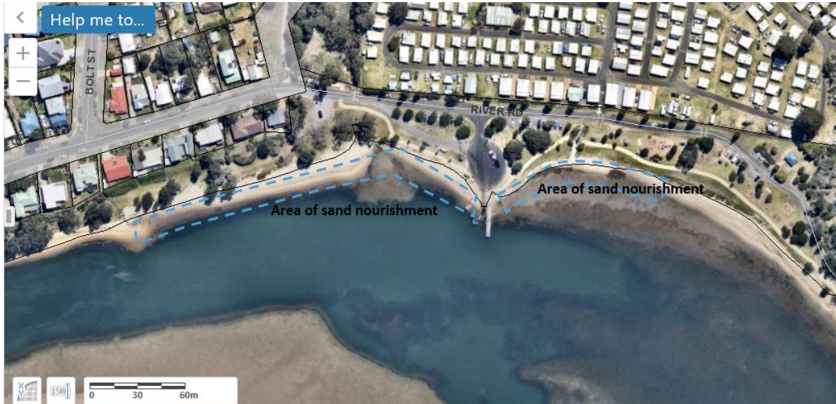
Figure 1: Area of northern foreshore that received 1000m 3 of sand nourishment from the Shoalhaven River flood notch maintenance work.
